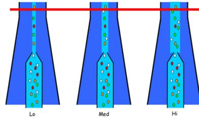
Each event that goes through the machine creates a pulse, with information about height, width and area of that pulse. Using this we can discriminate against doublets.
