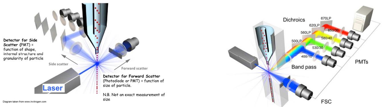
Filters separate the emitted fluorescent light into towards individual detectors. PMT (photomultiplier tube) = convert light energy into electrical voltage. PMT sensitivity can be increased/decreased by changing voltage on the cytometer software.
