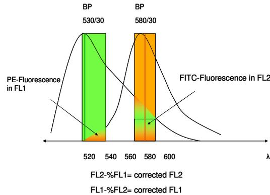
Every fluorescent molecule emits light with a particular spectrum unique to that molecule. To simultaneously measure the emissions from multiple fluorochromes, we can choose optical filters ("bandpass filters") which only transmit specific wavelengths of light. For simultaneous detection of emissions, whole spectra must be considered rather than only emission maxima. These emission spectra overlap for multiple fluorochromes, in some cases very significantly.
